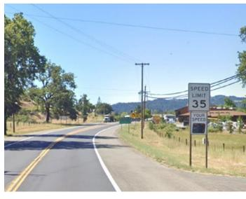
Figure 7-16: Speed Feedback Signs
